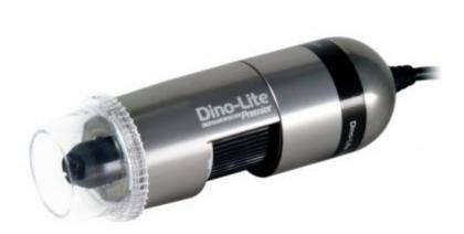
The Dino-Lite AM7013MZT4 has a 5 megapixel sensor for crystal clear images. With its high magnification of 400~470x, it reveals even the smallest details on all kinds of objects. The built-in adjustable polarizer reduces glare and reflection on shiny objects.
